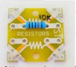
6 Use a marker to write the resistor Ohm value on Tile
