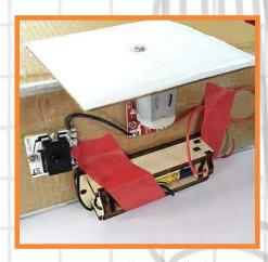
Cut a cardboard circle or square for spinner. This photo shows a screw on top, but you can just push the card onto the motor shaft.
