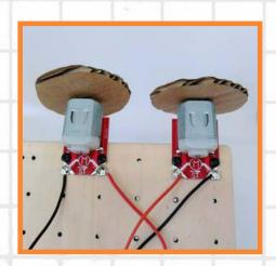
4. We've used the custom breadboard to screw the motors on for testing. You can use a cardboard box and screw or blutack the tiles on.
