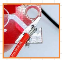
2. Firmly wrap 2cm wire around the corner of tiles. You can strip wires with a vege knife - see Technical Tips.
