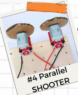
Why would you wire a circuit in parallel? It's so both motors get the full power or "push" from the battery, In a series circuit, they have to share it.
